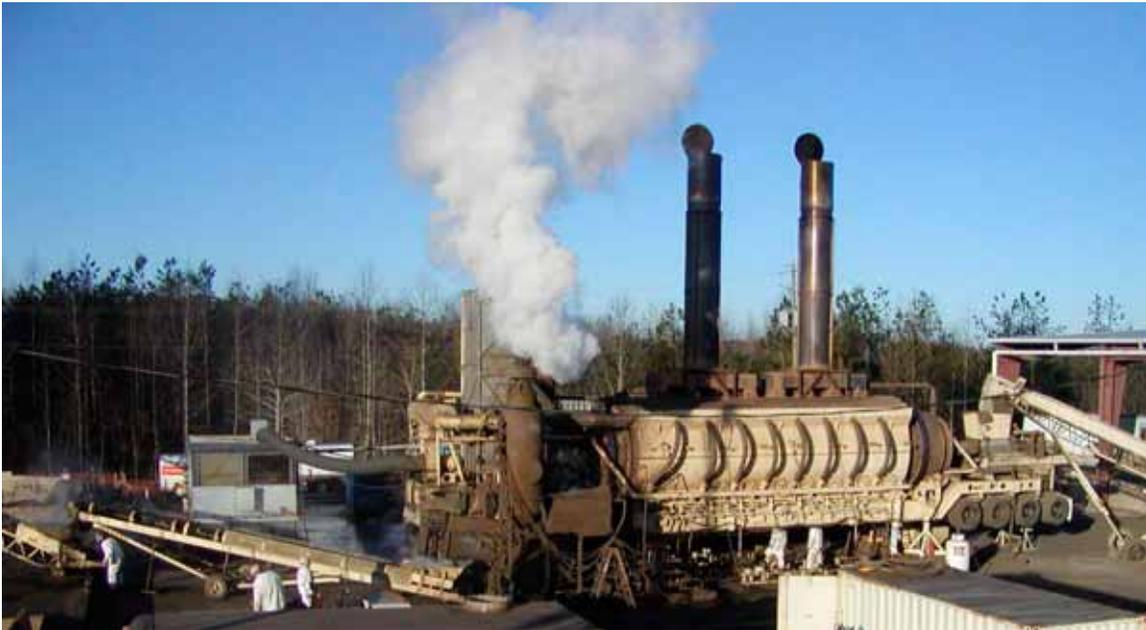
The project average PCB level in the treated soil was 0.137 ppm. The demonstrated system equivalent DRE for PCBs ranged from 99.999999% to 99.9999999% (i.e. “eight-nines” to “nine-nines”); 100 to 1000 times more efficient than required by the PCB treatment permit. Based on the results of the TSCA demonstration, USEPA is issuing a national mobile operating permit for the thermal desorption unit. About 4,500 gallons of concentrated PCB oil was condensed and recovered and ultimately disposed of.
